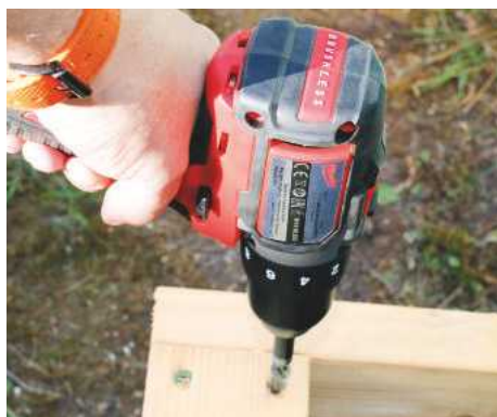
▲ Constructing some decking with 100 x 6mm screws was a breeze
